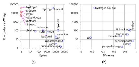
....and as you can see from graph (a). hydrogen holds a theoretical<sup>3</sup> 39kwh of energy per kilogram while a lithium battery holds about one tenth of a kWh per kg of battery. Hydrogen itself doesn't have a life cycle, but graph (a) shows that a hydrogen fuel cell lasts an order of magnitude longer in terms of throughput than a battery.
